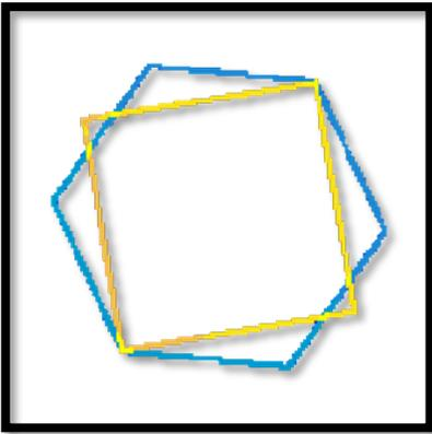
*“Order defines the number of corners on the polygon, which can range from a line (order 2) to an almost perfect circle (order 28) with all fractional settings in between. The number of corners defines the ratio of overtones with respect to the fundamental frequency: a low count keeps the harmonics near the fundamental frequency, a high order shifts them up.”*
