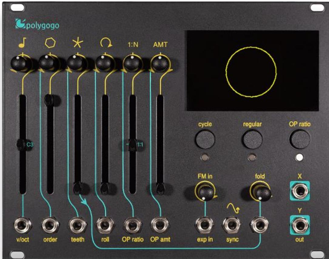
A graphical stereo oscillator with Polygonal Synthesis, originally invented at E-RM by Maximilian Rest and [Christoph Hohnerlein](#). Based on complex two dimensional amplitude shaping of sine waves, combined with internal modulation sources and a new type of wave folder.
