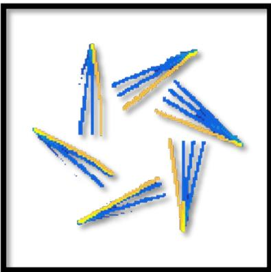
*“Teeth was the first happy accident while playing with the core formula of polygonal synthesis. It tilts the sides of the polygon out of the normal orientation and can be used to control the loudness of the overtones. It creates discontinuities in the waveform and acts as balance between the fundamental frequency and the overtone spectrum.”*
